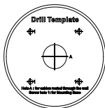
Figure 2-12 Drill Template of the Junction Box
