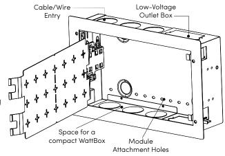
The back wall of the VersaBox Pro has holes and knockouts stamped into it on 6" centers for structured-can module installation. Use a 1/4" drill bit to widen the knockout stamps as needed.
