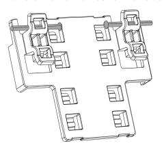
In addition, the standoffs have two clips to hold the central support plate: you can clip it toward the outside (left) or toward the inside (right).
