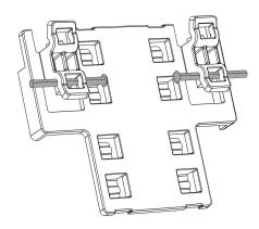
Finally, the central support plate can be inserted so that it curves toward the front of the enclosure, or recesses to the rear. Between the standoff orientation, the two clipping options, and the reversible support plate, this provides multiple depth options, up to being flush with the front of the enclosure.
