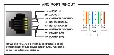
The Symetrix ARC-PSe provides serial control and power distribution over standard CAT5/6 cable for systems with more than 4 ARCs, or, when any number of ARCs are located long distances from a Integrator Series, Jupiter or Symetrix DSP unit.
