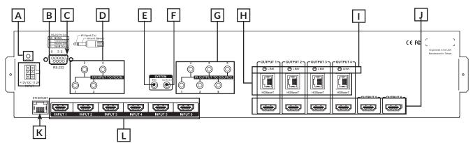
FIGURE 4: B-520-MTRX-230-6x4+2 Switcher Layout (Rear View)
