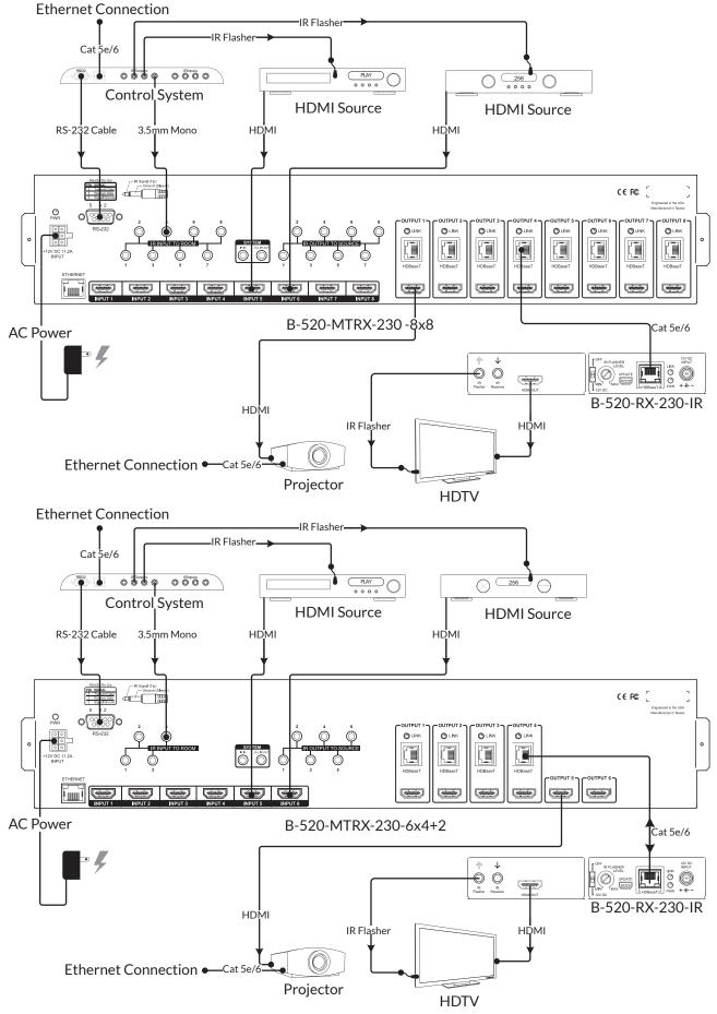
FIGURE 16: IR Passthrough Using Control System
