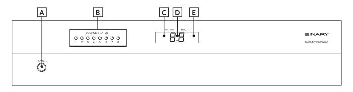
FIGURE 1: B-520-MTRX-230-8x8 Switcher Layout (Front View)
