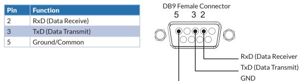
FIGURE 9: RS-232 (DB9) Pin Configurations
