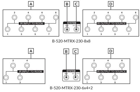
FIGURE 10: IR Connections
