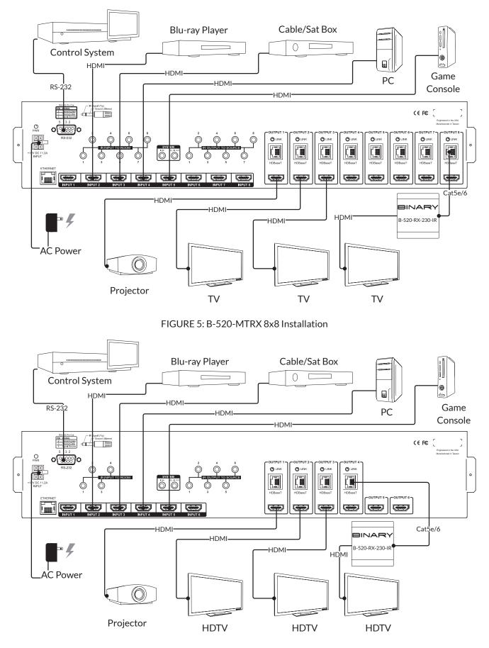
FIGURE 6: B-520-MTRX 6x4+2 Installation
