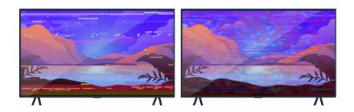
If the issue persists, define exactly what is wrong with the display. For example, mosaics and blocks, multiple lines or white dots, fixed horizontal, or vertical lines.
