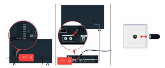
Check the antenna and input cable connections.
