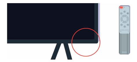
If the remote control sensor turns off when you press the power button, your TV is correctly connected to the power supply.
