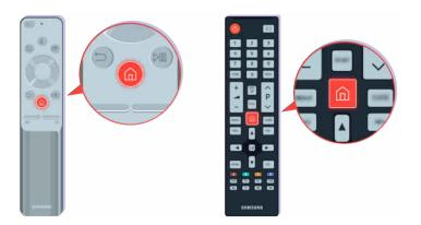
If there is sound but it is not clear, run a diagnostic test. On the remote control, press the **a** button.
