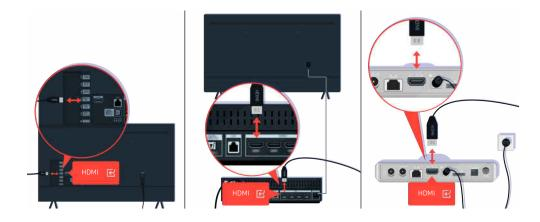
Check the antenna and HDMI cable connections.
