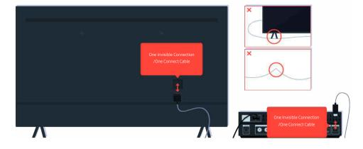
Disconnect and reconnect the One Invisible Connection or One Connect Cable between the TV and the One Connect Box. Make sure that the One Invisible Connection or One Connect Cable is not pinched or bent sharply.
