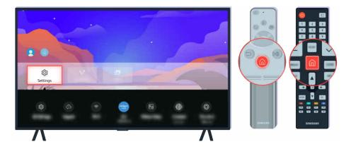
If the test shows no problems, select  $\textcircled{a} > \equiv Menu > \textcircled{s}$  Settings > Support > Device Care > Self Diagnosis > Broadcast Signal.
