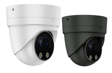
The 8MP Performance Series Turret Camera features a 4K Sony® Starvis™ sensor and includes a 2.7-13.5 mm motorized varifocal lens with autofocus. The camera supports IR night vision up to 25 meters, micro SD card support for local storage up to 512 GB, and features an IP67 rated housing to protect the camera from outside elements.
