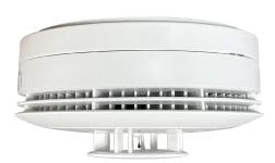
The ClareOne Smoke Detector is designed to quickly recognize problem smoke while decreasing false alerts from everyday cooking events. When the Smoke Detector's photoelectric (optical) sensor detects the presence of smoke, it sounds the alarm and then wirelessly transmits the information to the ClareOne Panel to further signal an alert. Meeting new UL standards (UL-268 and ULC-268), this Smoke Detector also employs a thermistor sensor to alert in instances of rapid heat rise.
