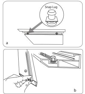
• The snap lugs line up with the arrow decals on the frame tubes. Alignment is not critical at this stage of the installation. Note that the screen is supplied with 2 extra snap lugs; should you lose or break a snap lug, one of the spares is a convenient replacement.
