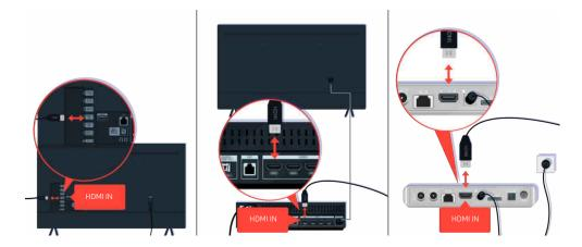
Check the antenna and HDMI cable connections.
