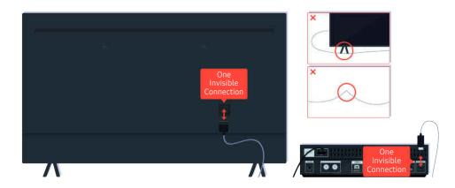
Disconnect and reconnect the One Invisible Connection cable between the TV and the One Connect (OC) Box. Make sure that the One Invisible Connection cable is not pinched or bent sharply.
