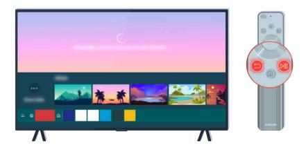
Press the  $\bigcirc$  and  $\bigotimes$  buttons simultaneously to display the pairing animation clip.
