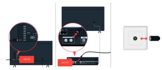
Check the antenna and input cable connections.
