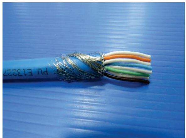
4. Cut away the shield layer and twist the drain wire for welding.
