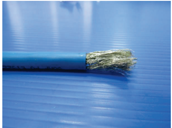
2. Strip the Category cable.
