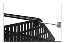
**Step 3 (Optional)** - Attach the top equipment brace(s) to the shelf sides using screws provided.
