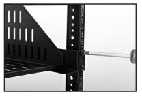
**Step 2 (Optional)** - Attach the rear support brackets to the rack frame using the supplied washers and screws.
