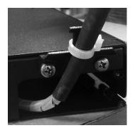
Secure feeder cable to cable entry clamp using supplied hose clamps or other suitable fastener like a zip-tie.
