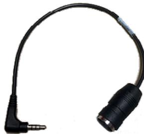
2. Attach the 4 conductor Din adapter to the speaker bar connector and then plug the 3.5mm plug inside the cable bay into the speaker bar output.
