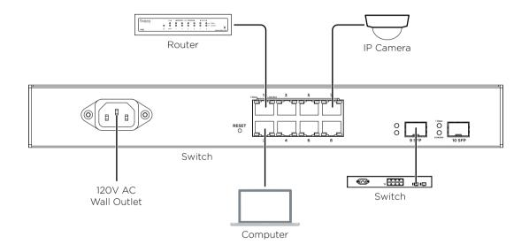
NOTE: Connect SFP ports using Araknis SFP adapters for RJ45 or multi-mode fiber cables. SFP adapters sold separately.
