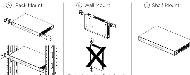
The switch must be wall mounted with the Ethernet ports facing either the floor or the ceiling.
