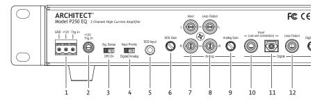
Master Trigger – This 3-pin block connector is used to turn on the unit or place it into standby mode. You can also use the 1/8" TS trigger to turn the unit on and off too. If no trigger voltage is present at either jack, then the unit will be in standby, with output muted.
