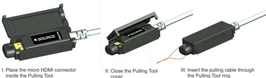
Figure 3: Attaching the Pulling Tool
