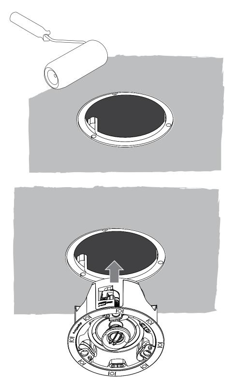
11. Install a round frameless grille (SKU: ESS-GLXRND-IC-X), which attaches magnetically to the speaker.
