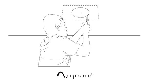
4. Fit the bracket into the opening and ensure it sits flat against the drywall.
