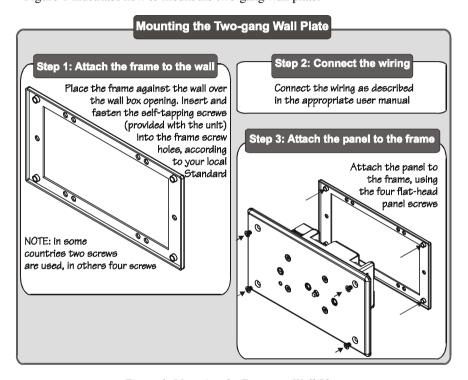
Figure 1: Mounting the Two-gang Wall Plate
