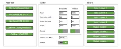
Figure 52: The Custom Resolutions Page - Current Parameters
