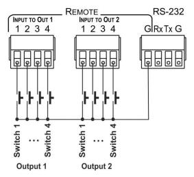
Figure 7: Remote Contact-closure Switch Connections
