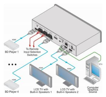
Figure 3: Connecting the VS-42UHD 4x2 HDMI Matrix Switcher
