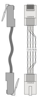
Figure 20: TP Pinout Wiring
