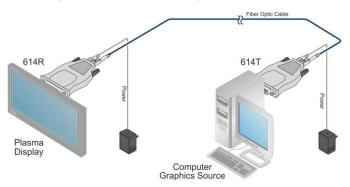
Figure 2: Connecting the 614T/614R
