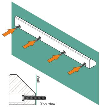
Figure 8: Installing the Bracket
