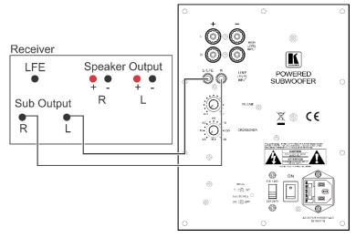
Figure 5: Connecting via Line Input
