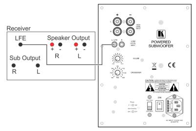
Figure 4: Connecting via LFE
