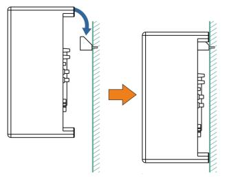
Figure 9: Mounting Tavor 8-Sub over the Bracket
