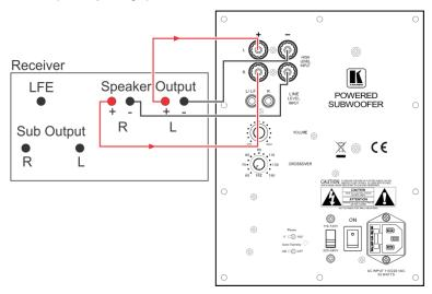
Figure 6: Connecting via High Level Input
