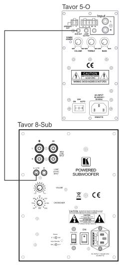
Figure 7: Connecting to an Active Speaker
