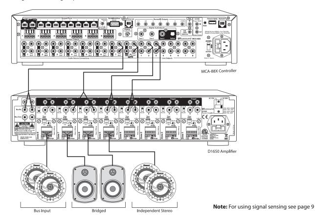
Connections for audio distribution preamp outputs
