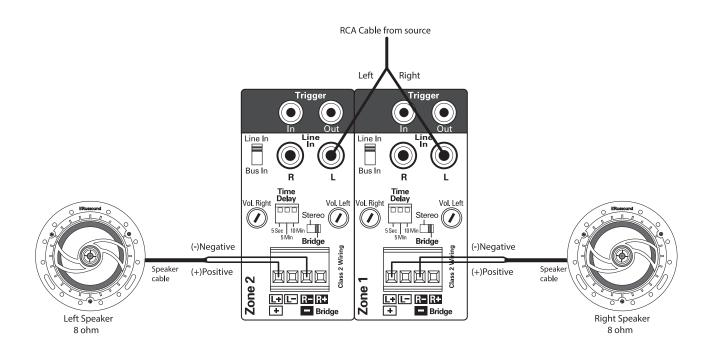
Connections for Bridge mode operation
