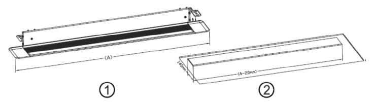
Measure the total width of the case (A) and subtract 20mm(3/4") for your hole length. The hole width will be 140mm(5 ½"). After you have identified your location and have measured twice you are now prepared to cut once.
