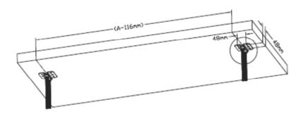
The distance between the center part of each ceiling bracket is (A) and subtract 116mm(4 ½"). The ceiling mounting bracket holes are placed 48mm(1 7/8") apart.
