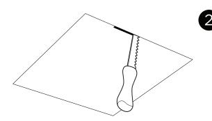
**Retro installation only:** Draw an outline around the template then remove the template, from ceiling. Follow the drawn lines to cut hole in drywall for the speaker.
