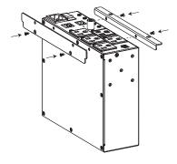
Open the knockout in the bottom of the VersaBox and install the enclosure. Insert the WattBox after the enclosure is installed.
