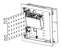
3. Fasten the brackets to the enclosure using 4 screws. (These screws are supplied with the enclosure.)
