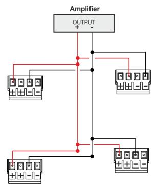
Figure 6: Array Layout Parallel Wiring
